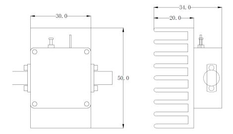
Including a small heatsink without Fan if output Power higher than +20dBm.
